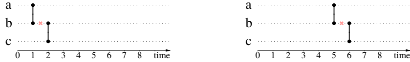
Figure 2: Two link streams illustrating the fact the impact of a shortest fastest path depends on the amount of temporal node pairs for which it is a shortest fastest path. Left: L = (T, V, E) with T = [0, 10] , V = \{a, b, c\} , and E = \{(1, ab), (2, bc)\} . The temporal node (1.5, b) is marked with a cross. Right: L = (T, V, E) with T = [0, 10] , V = \{a, b, c\} , and E = \{(5, ab), (6, bc)\} . The temporal node (5.5, b) is marked with a cross.
