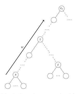
Figure 1: The PathLabel algorithm detects when vertex w on the path from s to the root  $v_r$  is an ancestor of the vertex z = LCA[s, t], without determining z.
