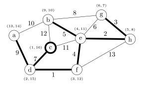
Figure 2: An example graph on 8 vertices  $(a, \ldots, h)$  and 13 weighted edges. The MST root vertex c and MST edges are highlighted by thicker lines.
