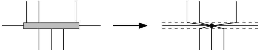
Figure 3: Converting a bar-drawing into a poly-line drawing.
