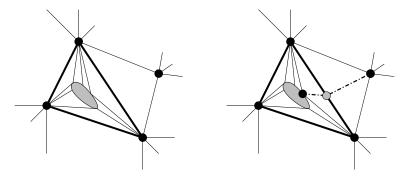
Figure 7: A separating triangle removed by subdividing one of its edges and re-triangulating.
