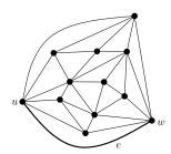
(a) A triangulated plane graph G; e is one of the edges of its outer-face.
