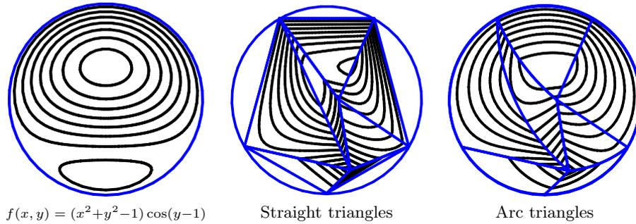
Figure 13: Approximation power of arc triangles versus straight triangles. The error for  $L^2$  drops from 0.18 (straight) to 0.07 (arc), and for  $L^{max}$  from 0.30 to 0.15.
