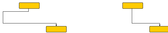
Figure 5: An edge that is a bow (left) and the edge after bow reduction (right).
