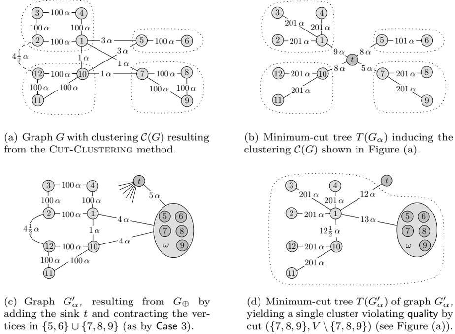
Figure 2: Counter-example for the correctness of Case 3.
