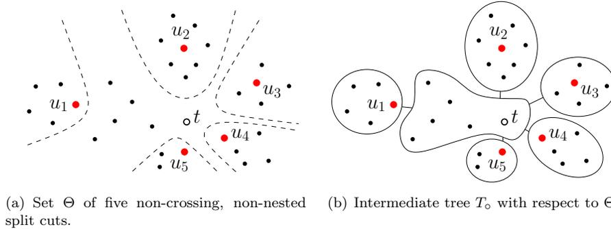
Figure 6: This example shows an intermediate minimum-cut tree  $T_\circ$  regarding vertices  $u_1, \dots, u_5$  (b); in order to have  $T_\circ$  define a clustering, the vertices inside  $t$ 's super-node need to be separated from  $t$  by further cuts.
