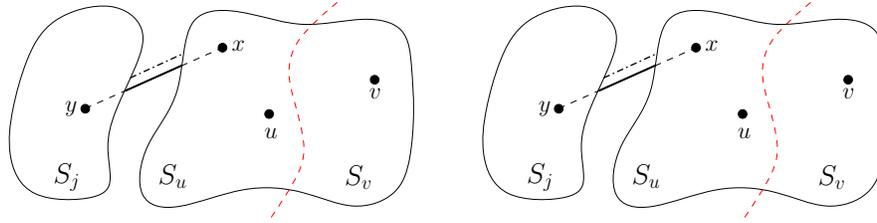
(a) If  $x \in S_u$  vertex pair  $\{x, y\}$  remains a cut pair of edge  $\{S_u, S_j\}$  in  $T_*$ . (b) Although  $x \notin S_u$ , with  $\{u, y\}$  there is still a cut pair in the adjacent nodes  $S_u$  and  $S_j$  in  $T_*$ .
