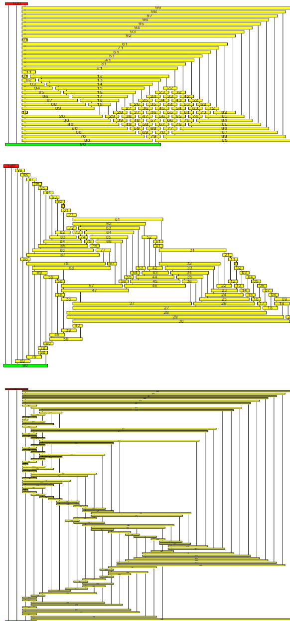
Figure 12: Visibility representations of a 10 \times 10 grid graph for different st -orientations produced with \text{PAR-STN}(p) ( p = 0, 0.25, 1 ). The respective areas (height \times width) are 35 \times 34 = 1190 , 46 \times 50 = 2300 and 99 \times 34 = 3366 .
