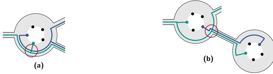
Figure 9: The two cases how \mathbf{t}/\mathbf{t} -crossings in O-drawings can arise: In (a) , the blue tracks orbit inside the green ones, thus causing a crossing when they pass the green vertex. \mathbf{t}/\mathbf{t} -crossings are highlighted with the red circles. The crossing in (b) occurs because the green track blocks the visibility to the lower-right disk for the blue track. Observe that there is only one \mathbf{t}/\mathbf{t} -crossing in (a) , although there is technically one blue track from the upper- and one from the lower-right disk.
