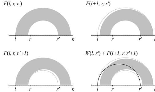
Figure 3: A diagrammatic representation of our algorithm. The diagrams correspond to the terms in the dynamic programming recurrence defined in Equation 1. The grey half-annulus represents an optimal clique such that all left endpoints are in the left range, and all right endpoints are in the right range. The initial extent of the half-annulus is represented by grey arcs; this is to help illustrate a change in half-annulus ranges. Arcs newly added to the clique are denoted by a darker arc.
