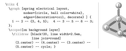
Figure 3: Example of a picture where the graph drawing system is used to first render a six node graph using a spring electrical layout. Subsequently, the positioned nodes can be referenced normally such as in the code that adds the shaded area on the background.
