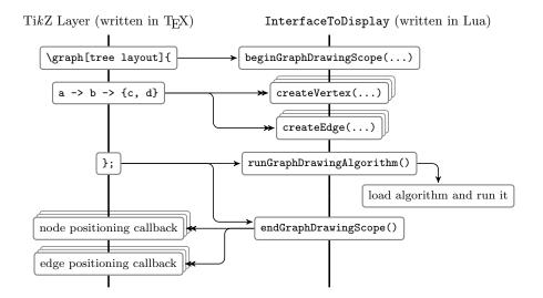
Figure 2: Call graph of the interaction between TikZ and the interface of the framework. Naturally, this figure has been created using graph drawing in TikZ: The Sugiyama method was applied to the call graph and same layer was used with all node pairs that needed to be aligned horizontally. For the edges between nodes on different layers, TikZ's capability of rendering edges using only horizontal and vertical segments was harnessed.
