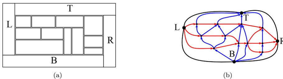
Figure 1: (a) A rectangular dual; and (b) its transversal structure.
