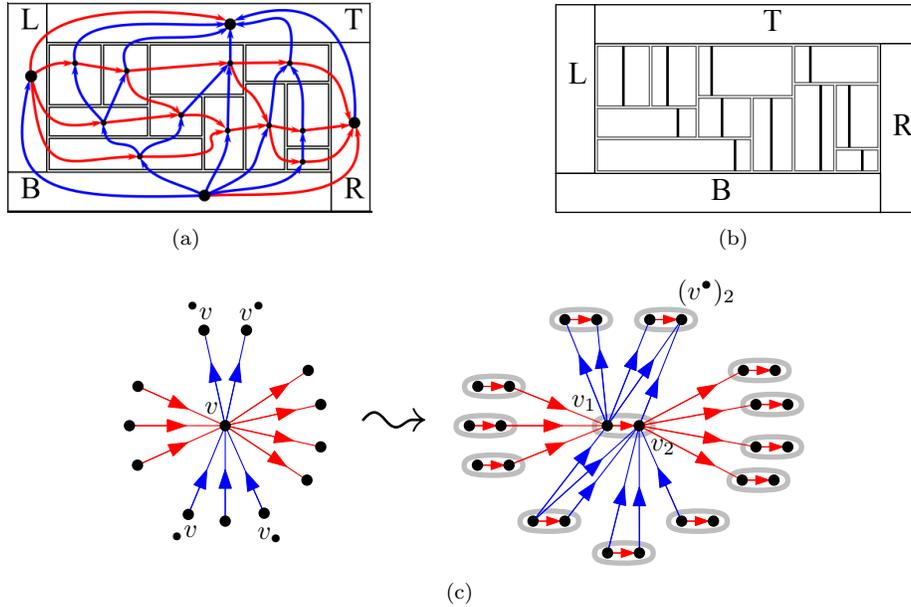
Figure 3: (a) The minimal rectangular dual of the graph in Fig. 1 with its transversal structure overlaid on it. (b) A rectangular dual of the split graph of (a). (c) Splitting a vertex  $v$  into  $v_1$  and  $v_2$  and the corresponding transversal structure.
