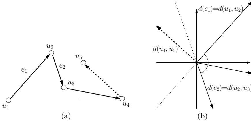
Figure 4: (a) A path  $P(u_1, u_4)$  and an edge  $(u_4, u_5)$  whose direction is in  $opp(P(u_1, u_4))$ . (b) There exists no wedge having an angle smaller than  $\pi$  containing all of  $d(e_1)$ ,  $d(e_2)$ , and  $d(u_4, u_5)$ .
