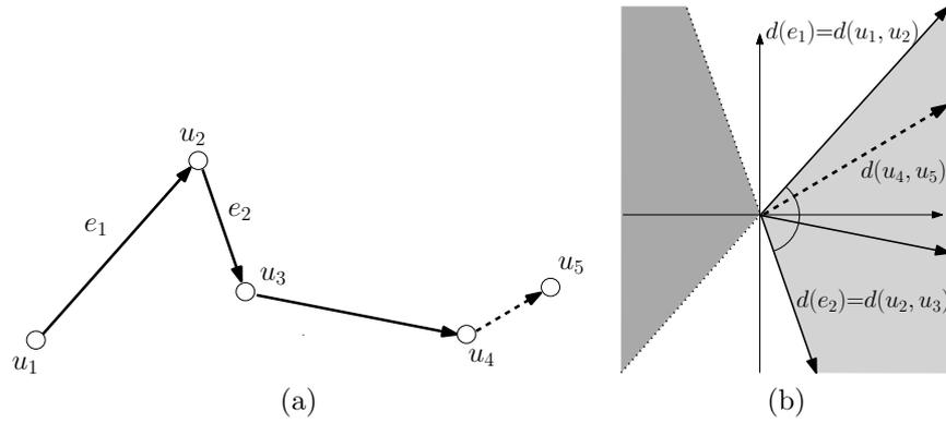
Figure 5: (a) A path  $P(u_1, u_4)$  and an edge  $(u_4, u_5)$  whose direction is in  $\text{range}(P(u_1, u_4))$ . (b)  $\text{range}(P(u_1, u_4)) = \text{range}(P(u_1, u_5))$ .
