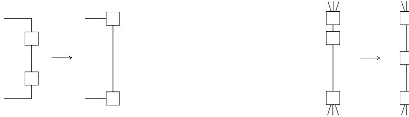
Figure 8: Refining poor placement of degree two nodes. The illustration on the left shows the movement of degree two nodes to remove bends while the right demonstrates a node placement with better distribution.
