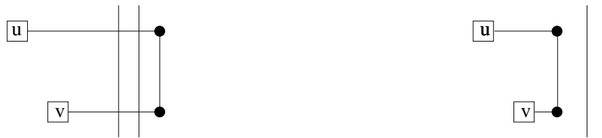
Figure 3: Fixing a U-Turn edge. The left illustration shows the nodes and edges in their original positions. The endpoints of the middle segment are shown with circles and the source and target of the U-Turn with boxes. The right illustration shows the final placement.
